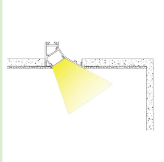
Trimless recessed wall washer profile with opalised diffused cover.
