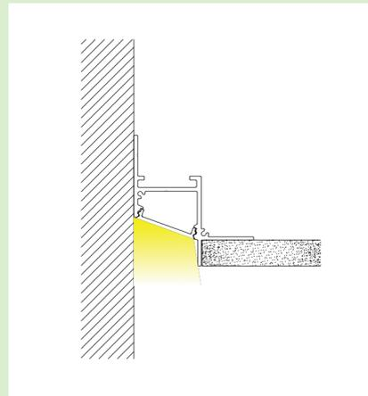
Corner recessed wall washer profile with opalised diffused cover.
