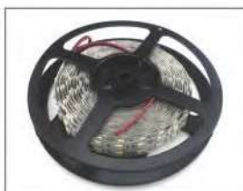
LED Strip: 3528LED, 240LEDs/M, 19.2W/M, double rows
